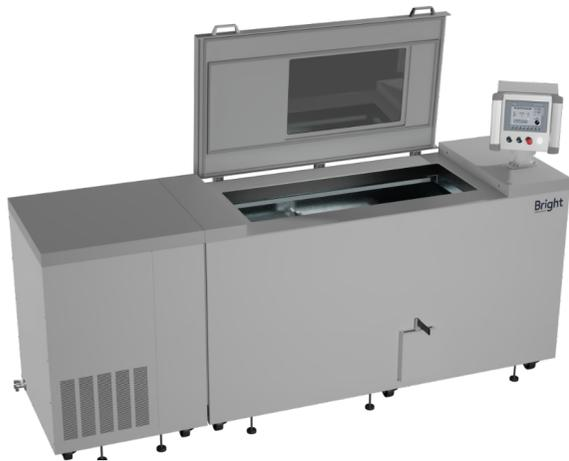
**Caution:** Before lifting the large access lid, please ensure the smaller glass lid is closed and locked into position.
