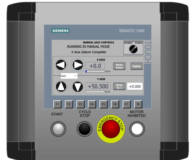
The X axis value should read +0.0 when at datum point.
