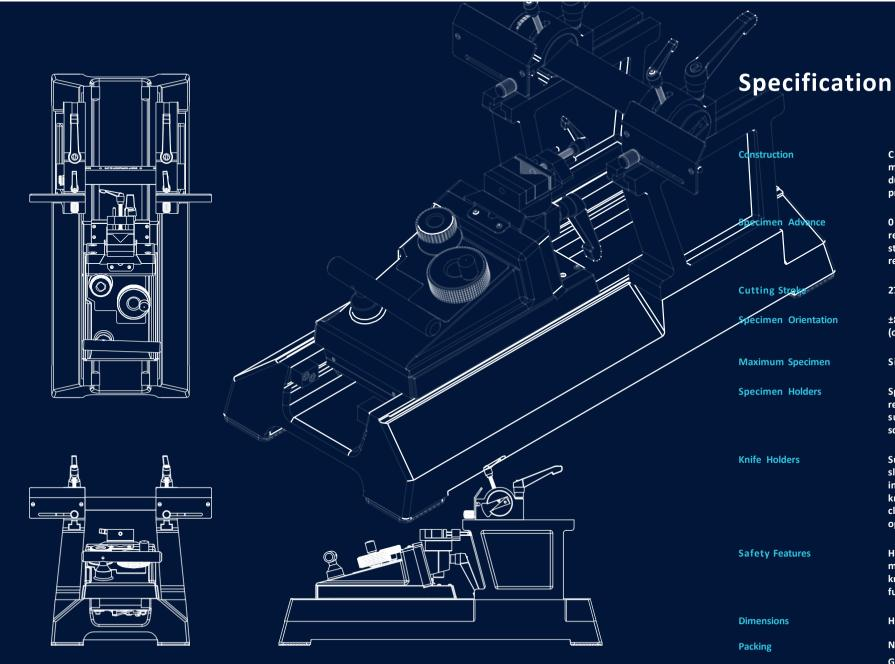
Cast mechanite, precision machined and fi nished with durable solvent and detergent proof coating
