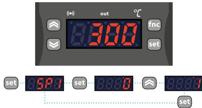
Once the 'SP1' label has been displayed, press the "set" button to display the Set point 1 value. The Set point value appears on the display. To change the Set point value, use the "UP" and "DOWN" buttons within 15 seconds.
