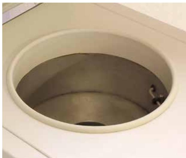
The lower chamber is pictured here containing the aluminium block for quick freezing.
